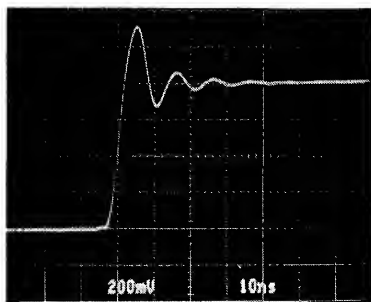
FIGURE 4. Output response of a real LM6181, A_V = +2 , R_f = R_g = 820\Omega . Output load is oscilloscope probe, Tektronix P6106A, 10 M \Omega , 8.7 pF.
