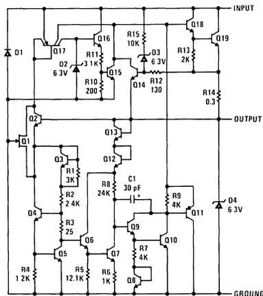
Figure 3. Detailed Schematic of The Regulator.
