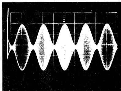
FIGURE 25. 455 kHz Modulated by 100 Hz
