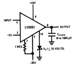
Figure 6A. LH0001 As Comparator For Driving MOS.
