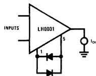
Figure 9. Method of Reducing Output Short Circuit Current.
