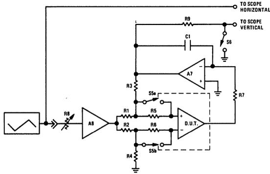
FIGURE 1. Functional Diagram of Bias Current Test Circuit
