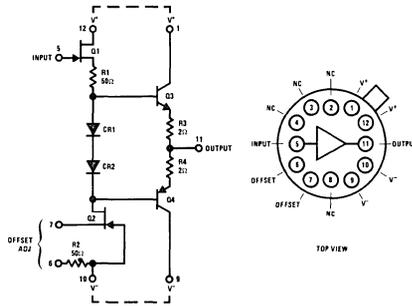
FIGURE 2. LH0033 Schematic
