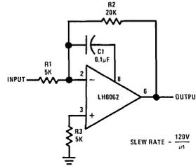
FIGURE 5. Feed Forward Compensation
