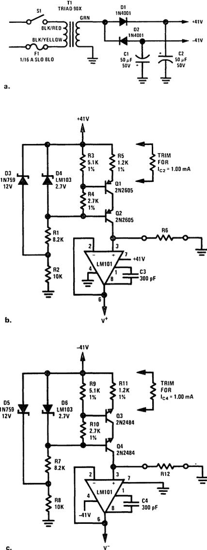
FIGURE 28. Low-Power Supply for Integrated Circuit Testing
