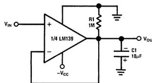
FIGURE 43. Negative Peak Detector
