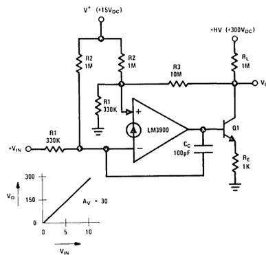
FIGURE 94. A High Voltage Non-inverting Amplifier
