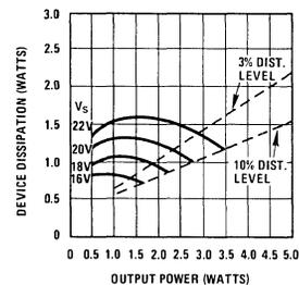
FIGURE 3C. Device Dissipation vs Output Power – 16Ω Load
