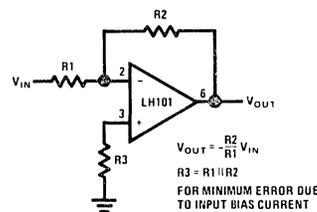
FIGURE 1. Inverting Amplifier
