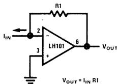
FIGURE 13. Current to Voltage Converter
