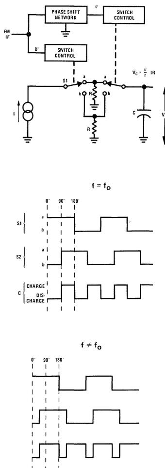
FIGURE 7. Quadrature Detector Analog and Timing Diagrams
