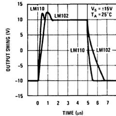
Large signal pulse response shows 40V/µs slew for LM110 and 10V/µs for LM102. Leading edge overshoot on LM110 is virtually eliminated, so external clamp diode frequently required on the LM102 is not needed.
