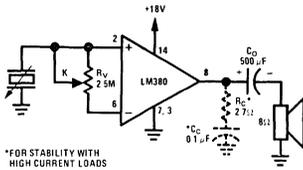
FIGURE 9. "Common Mode" Volume Control
