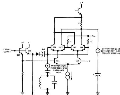
FIGURE 8. Simplified Equivalent Circuit of Quadrature Detector
