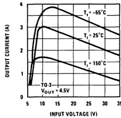
Figure 4. Current-Limiting Characteristics.
