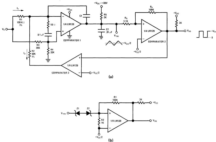
FIGURE 17. Voltage Controlled Oscillator
