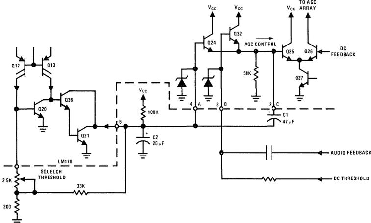
FIGURE 28. Simultaneous Squelch and AGC
