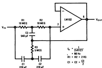
FIGURE 1. High Q Notch Filter
