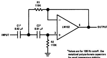
\*Values are for 100 Hz cutoff. Use metallized poly-carbonate capacitors for good temperature stability.
