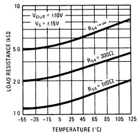
FIGURE 11. Minimum Load Resistance for Rated Output Swing
