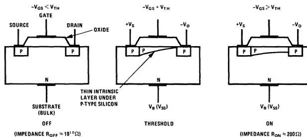
FIGURE 3. Channel Enhancement in MOS Transistors (P Channel)
