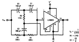
FIGURE 19. 4.5 MHz Notch Filter
