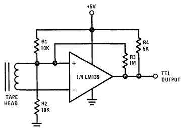
FIGURE 38. Magnetic Tape Reader with TTL Output
