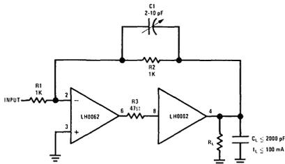
Note: In the examples above, a small capacitor,  $C_1$ , is used to cancel the effects of stray capacitance at the input.
