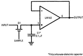
FIGURE 23. Sample and Hold Circuit
