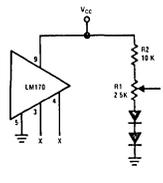
FIGURE 29B. Temperature Compensating Circuitry
