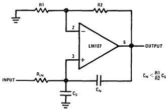
Neutralizing Input Capacitance to Optimize Response Time
