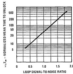
FIGURE 11. Unlock Behavior of High-Gain, Second-Order Loop,  $\zeta = 0.707$
