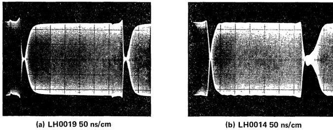
FIGURE 10. Channel Switching—LH0019 vs LH0014
