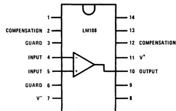
NOTE: Pin 7 connected to bottom of package.
