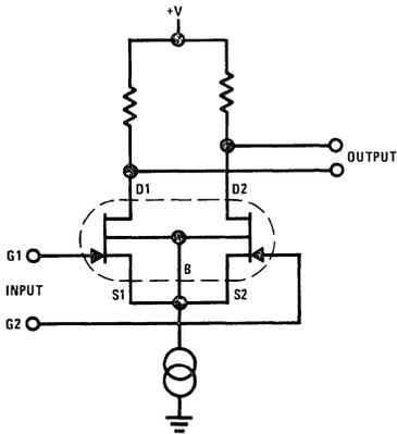
FIGURE 8. Large Common Mode Range Biasing, Common Source.
