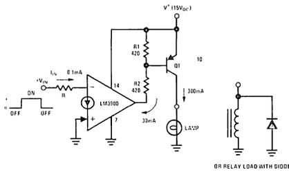
FIGURE 91. Boosting to 300 mA Loads
