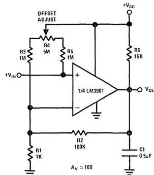
FIGURE 31. Input Offset Null Adjustment
