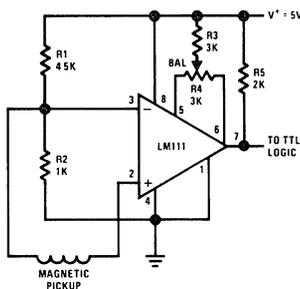
**FIGURE 2. Zero Crossing Detector for Magnetic Transducer**
