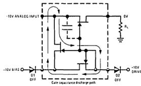
FIGURE 4. AM1000 Turning On
