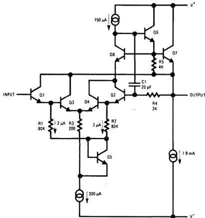
FIGURE 2. Partial Schematic of the LM102 Voltage Follower
