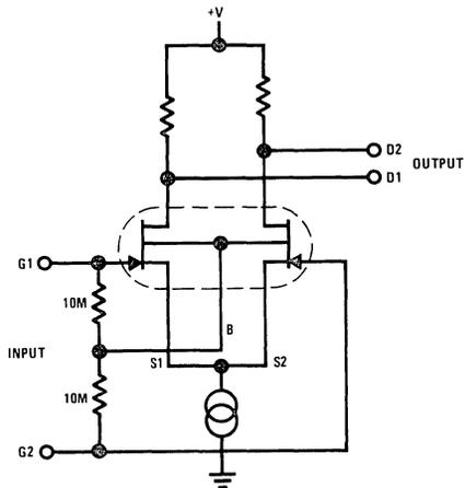
FIGURE 10. Best Biasing for Large Input Signals.
