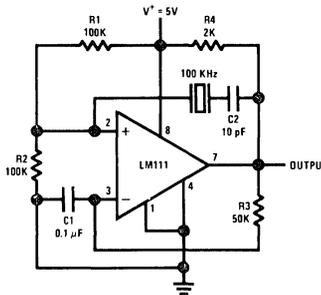
FIGURE 9. Crystal-Controlled Oscillator
