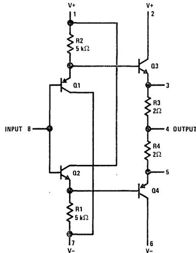
FIGURE 1. Circuit Schematic
