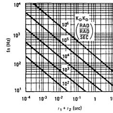
FIGURE 4. Filter Time Constant vs Natural Frequency
