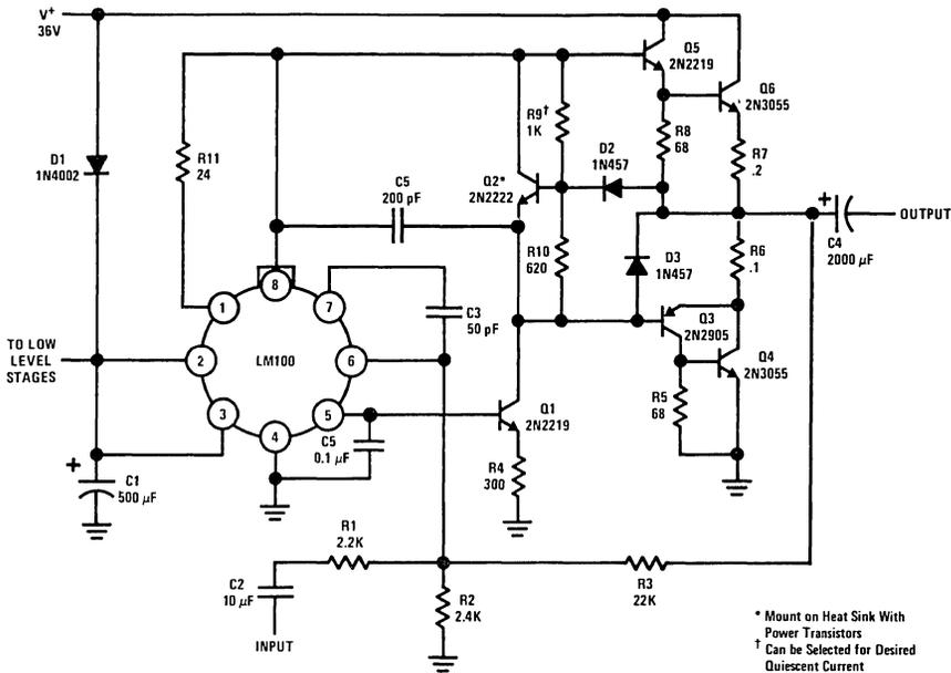
FIGURE 9. Power Amplifier With Current Limiting
