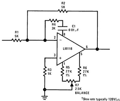
FIGURE 3. Feedforward Compensation for Greater Inverting Slew Rate†
