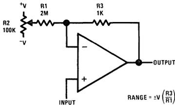
FIGURE 4. Offset Voltage Adjustment for Voltage Followers
