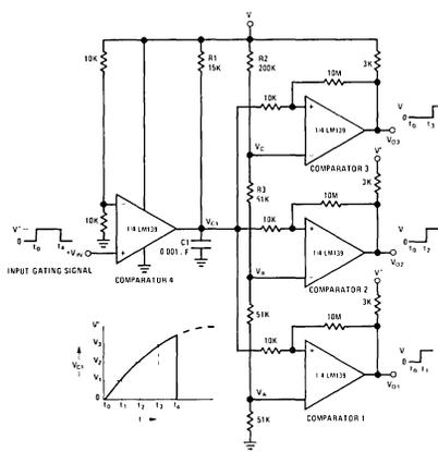
FIGURE 27. Time Delay Generator
