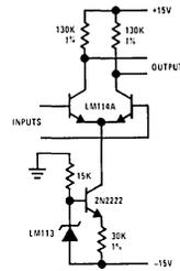
FIGURE 7. Amplifier Biasing for Constant Gain with Temperature
