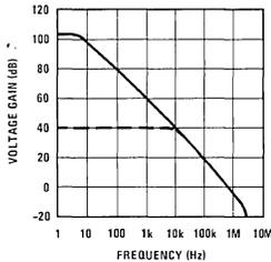
FIGURE 1. Open and Closed Loop Frequency Response
