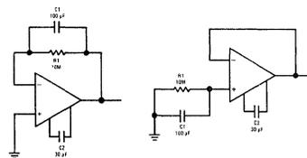
**FIGURE 7. Test Circuits for Selecting Bias-Compensation Resistors.**
