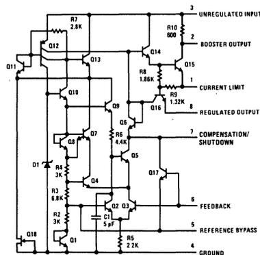
FIGURE 4. Schematic Diagram of the LM105 Regulator.
