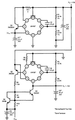
FIGURE 20. Positive and Negative Regulators using the LM100
