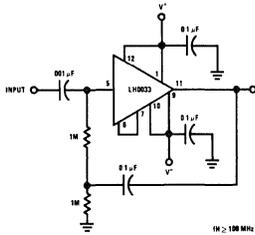
FIGURE 17. High Input Impedance AC Coupled Amplifier
