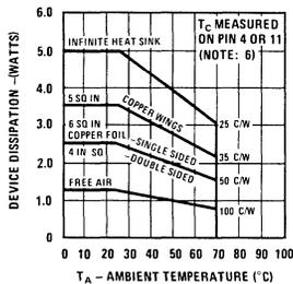
FIGURE 2. Device Dissipation vs Maximum Ambient Temperature
