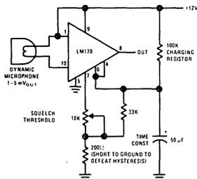
FIGURE 17. Squelched Preamplicifier with Hysteresis
