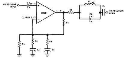
FIGURE 16. Tape Recording Preamp.
