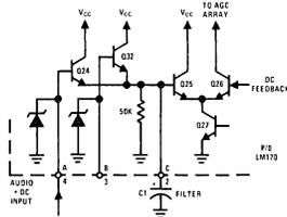
FIGURE 26. Internal AGC Control Circuitry
