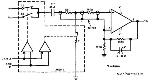
FIGURE 25. Precision Subtractor for Automatic Test Gear
