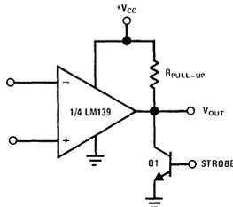
FIGURE 21. Output Strobing Using a Discrete Transistor
