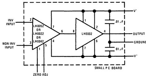
FIGURE 27. 100 mA Output FET Op Amp "Module"
