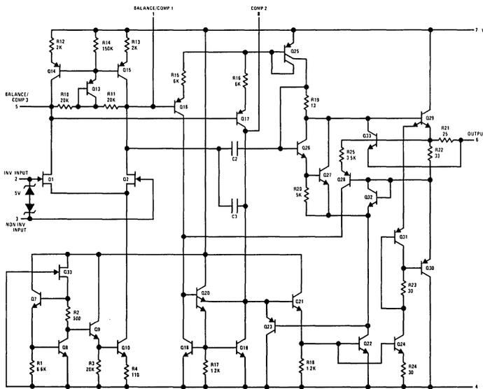
FIGURE 2. Complete LH0062 Schematic
