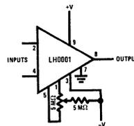
Figure 7. Method of Balancing Input Offset Voltage.
