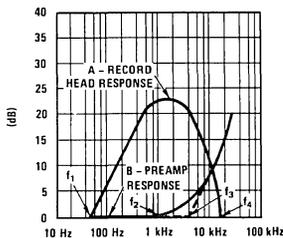
FIGURE 15. Recording Head & Preamp. Response for NAB Equalization
