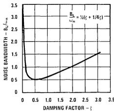
FIGURE 10. Loop-Noise Bandwidth (For High-Gain, Second-Order Loop)
