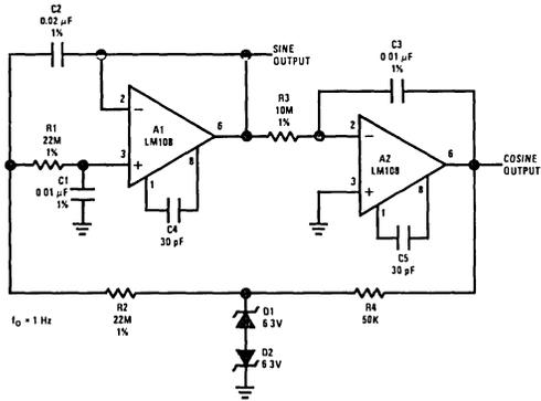
Low Frequency Sine Wave Generator with Quadrature Output
