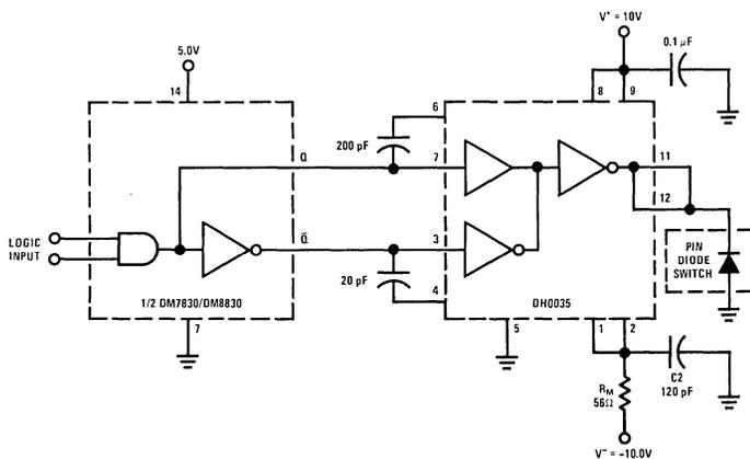
FIGURE 5. Anode Grounded Design
