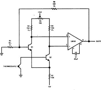
FIGURE 8. Example of a DC Amplifier Using the Drift-Compensation Technique.
