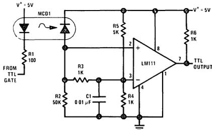
FIGURE 7. Data Transmission System with Near-Infinite Ground Isolation
