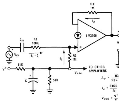
FIGURE 13. Non-inverting AC Amplifier Using Voltage Reference Biasing
