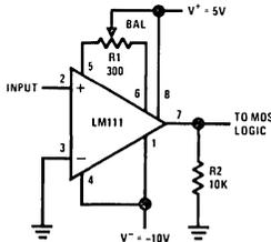
FIGURE 5. Zero Crossing Detector Driving MOS Logic
