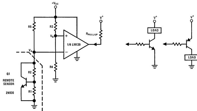
FIGURE 35. Temperature Alarm
