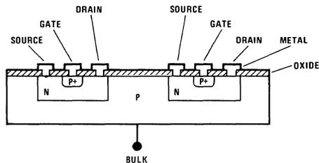
FIGURE 11. Simplified Cross Section of Monolithic JFET Dual.
