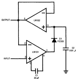
FIGURE 7. Positive Peak Detector with Buffered Output
