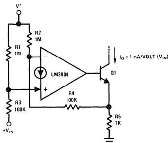
FIGURE 74. A Voltage Controlled Current Sink
