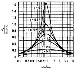
FIGURE 6. Steady-State Peak Phase Error Due to Sinusoidal FM (High-Gain, Second-Order Loop.)
