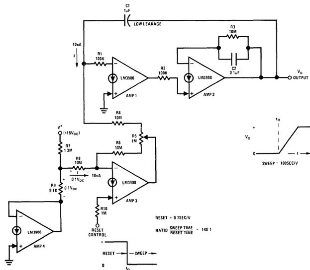
FIGURE 46. Generating Very Slow Sawtooth Waveforms
