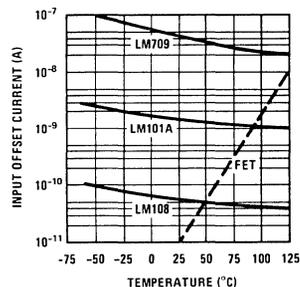
FIGURE 1. Comparing IC Op Amps With FET-Input Amplifier
