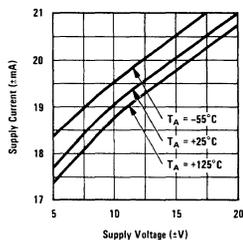
FIGURE 9. Supply Current vs Supply Voltage
