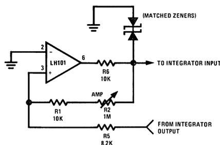
FIGURE 26. Threshold Detector with Regulated Output
