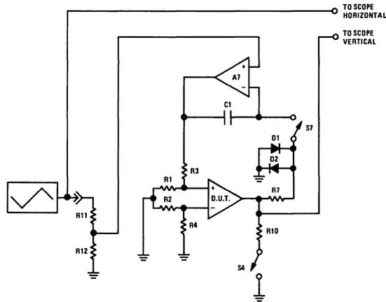
FIGURE 4. Functional Diagram of Transfer Function Circuit
