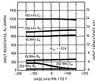
FIGURE 10. Effect of AGC on Cascode Input Impedance
