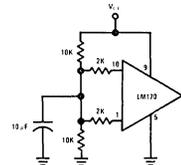
FIGURE 10. Input Biasing and Decoupling Network
