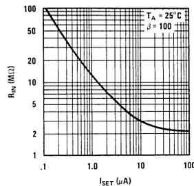
FIGURE 2. Input Resistance vs I<sub>SET</sub>
