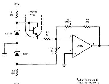
FIGURE 8. Electronic Thermometer
