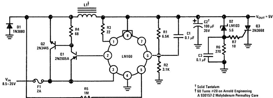
FIGURE 4. Switching Regulator with Crowbar Overvoltage Protection
