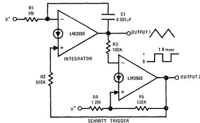
FIGURE 44. A Triangle Waveform Generator
