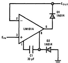
FIGURE 1. Precision Diode
