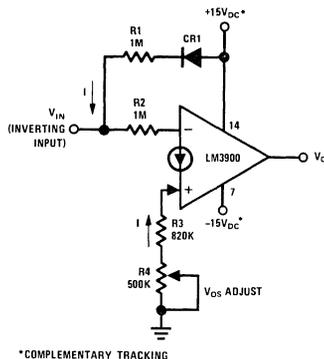
FIGURE 76. DC Biasing for  $\pm 15\text{ V}_{\text{DC}}$  Operation
