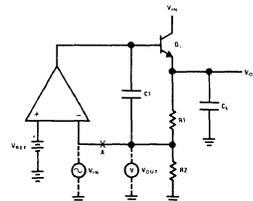
FIGURE 5. Simplified Schematic Showing Regulator Frequency Compensation
