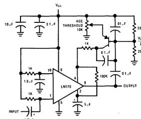
FIGURE 15. AGC Circuit with External Peak Detector
