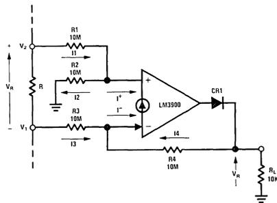
FIGURE 24. Ground Referencing a Differential Input DC Voltage
