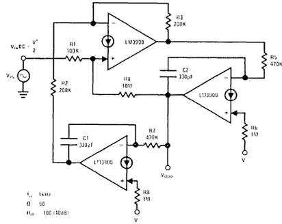
FIGURE 40. The "Bi-quad" RC Active Bandpass Filter
