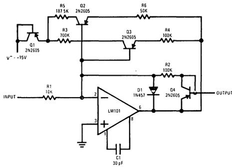
FIGURE 8. Nonlinear Operational Amplifier with Temperature-Compensated Breakpoints
