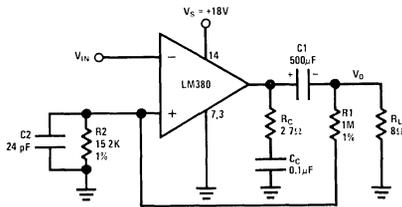
FIGURE 21. Boosted Gain of 200 Using Positive Feedback
