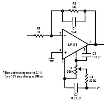
†Slew and settling time to 0.1% for a 10V step change is 800 ns
