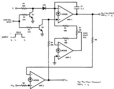
FIGURE 86. Sample-hold and Compare with New  $+V_{IN}$
