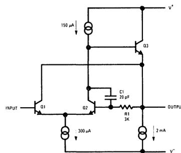
FIGURE 1. Basic Configuration of the Voltage Follower
