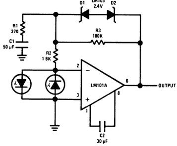
Saturating Servo Preamplifier with Rate Feedback
