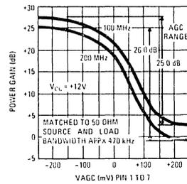
FIGURE 9. Tuned Cascode Power Gain vs AGC
