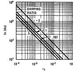
FIGURE 5. Damping Time Constant vs Natural Frequency
