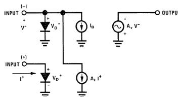
FIGURE 8. An Equivalent Circuit of the "Norton" Amplifier
