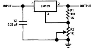
Figure 9. Using The LM109 As An Adjustable-Output Regulator.
