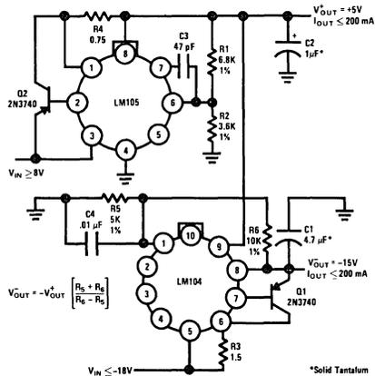
FIGURE 4. Tracking Regulators With Different Output Voltages
