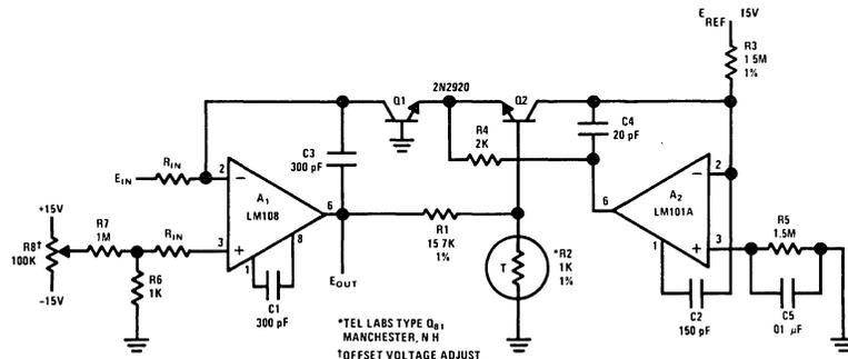
FIGURE 1. Log Generator with 100 dB Dynamic Range
