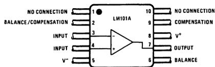
NOTE: Pin 5 Connected to bottom of package.
