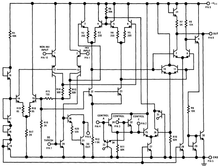
FIGURE 3. LM170 Schematic
