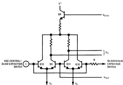
FIGURE 4. Attenuator Circuitry
