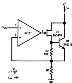
$$I_o = \frac{V_{IN}}{R_1}$$
