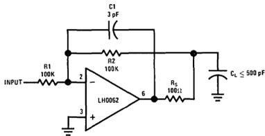
FIGURE 3. Isolating a Capacitive Load up to 500 pF
