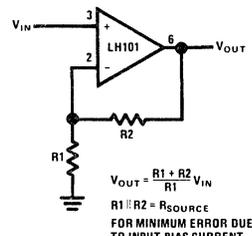
FIGURE 2. Non-Inverting Amplifier
