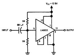
FIGURE 18. Single Supply AC Amplifier
