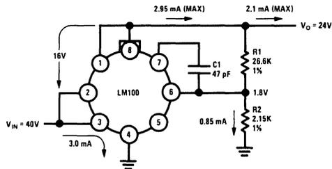
FIGURE 1. Circuit Used in the Solution of Question 1.
