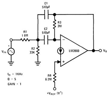
FIGURE 38. A One Op Amp Bandpass Filter
