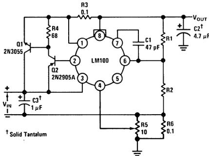
**FIGURE 14. Line Resistance Compensator for High Current Regulators**
