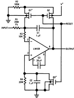
\* Q1 and Q3 should not have internal gate-protection diodes
