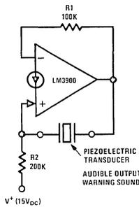
FIGURE 92. Positive Feedback Power Oscillators
