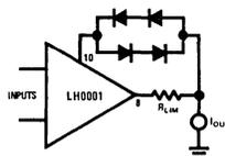
Figure 11. Alternate Method of Limiting Output Short Circuit Current.
