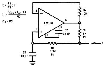
FIGURE 19. Capacitance Multiplier
