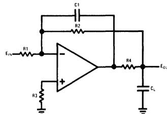
FIGURE 15. Compensating for Very Large Capacitive Loads
