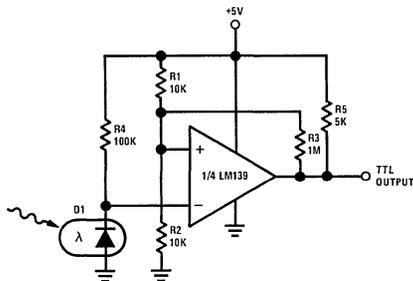
FIGURE 39. Paper Tape Reader With TTL Output
