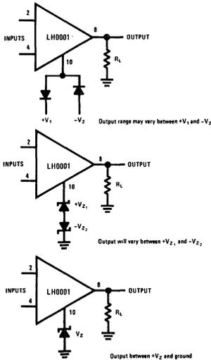
Figure 4. Methods of Restricting Output Voltage Swing.
