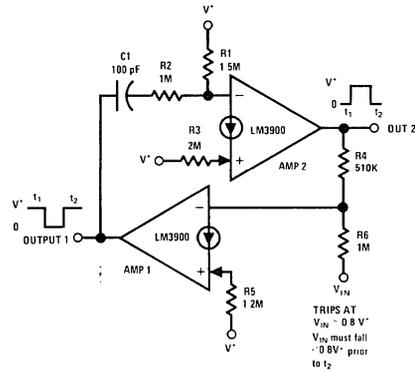
FIGURE 63. A One-shot Multivibrator with an Input Comparator
