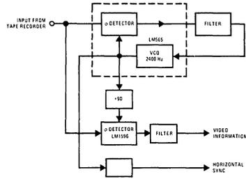
FIGURE 21. Block Diagram of Weather Satellite Demodulator
