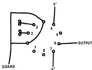
FIGURE 10. TO-5 - 10 Pin Pattern PC Layout
