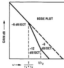
FIGURE 3. Phase Locked Loop with Damping Resistor Added
