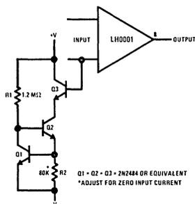
Figure 8. Method of Compensating for Input Bias Current.
