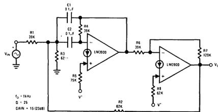
FIGURE 39. A Two Op Amp Bandpass Filter
