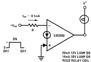
FIGURE 90. Sinking 20 to 30 mA Loads
