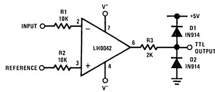
FIGURE 22. Precision Voltage Comparator
