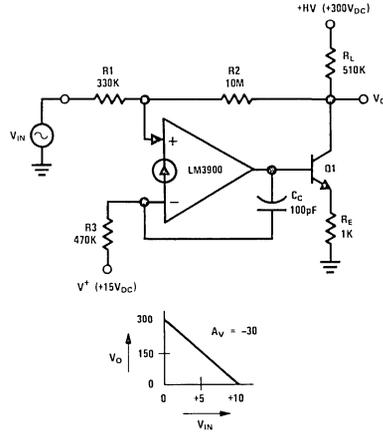
FIGURE 93. A High Voltage Inverting Amplifier
