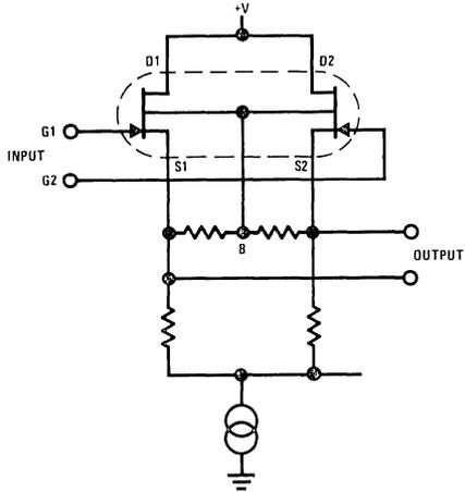
FIGURE 9. Large Common Mode Range Biasing, Common Drain.
