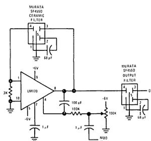
FIGURE 24. 455 kHz Modulated Constant Output Oscillator
