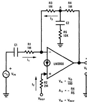
FIGURE 16. A High Z<sub>IN</sub> High Gain Inverting AC Amplifier
