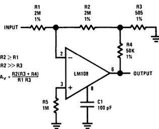
FIGURE 26. Inverting Amplifier With High Input Resistance
