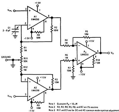
FIGURE 15.  $\times 100$  Instrumentation Amplifier
