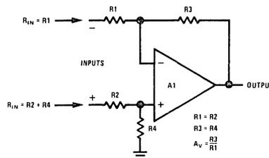
FIGURE 20. Feedback Connection For a Differential Amplifier
