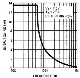
FIGURE 9. Frequency Limited Output Swing
