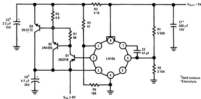
FIGURE 12. 10A Regulator with Foldback Current Limiting.
