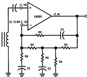
FIGURE 12. Two-Pole Fast Turn-On NAB Tape Preamp.
