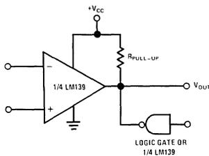
FIGURE 22. Output Strobing with TTL Gate
