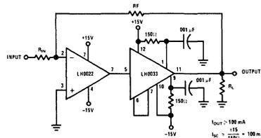
FIGURE 20. Using LH0033 as an Output Buffer
