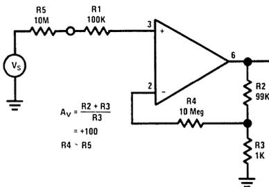
FIGURE 17. Non-Inverting Amplifier
