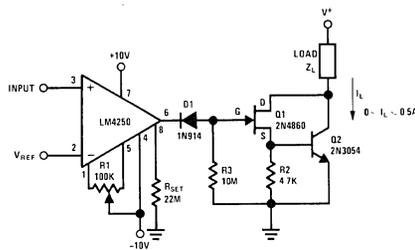
FIGURE 8.  $\mu$ -Power Comparator with High Current Switch
