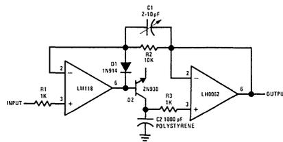
FIGURE 9. High Speed Peak Detector
