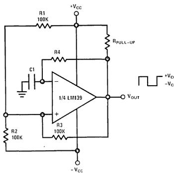
FIGURE 33. Squarewave Generator Using Dual Supplies
