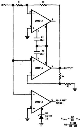
Absolute Value Amplifier with Polarity Detector
