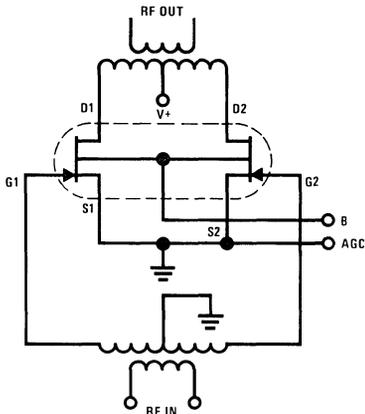
FIGURE 4. AGC Connections for Frequencies to 30 MHz.
