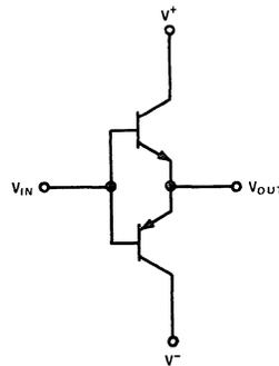
FIGURE 6. Simple Booster Amplifier
