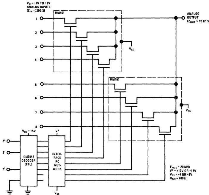
FIGURE 2. Hybrid MOS/TTL 20-MHz Commutator for Low-Level Signals
