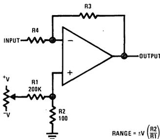
FIGURE 2. Offset Voltage Adjustment for Inverting Amplifiers Using Any Type of Feedback Element
