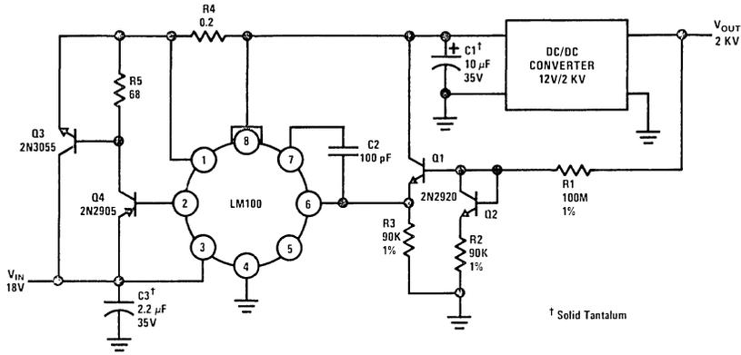
FIGURE 12. High Voltage Regulator
