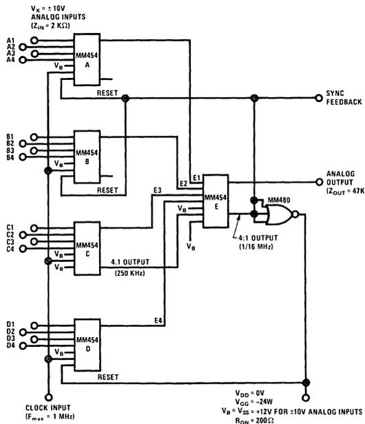
FIGURE 1. All-MOS 1-MHz Multiplexer or Commutator
