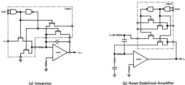
FIGURE 5. Switching Applications With Linear Circuits
