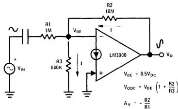
FIGURE 14. Inverting AC Amplifier Using N V<sub>BE</sub> Biasing
