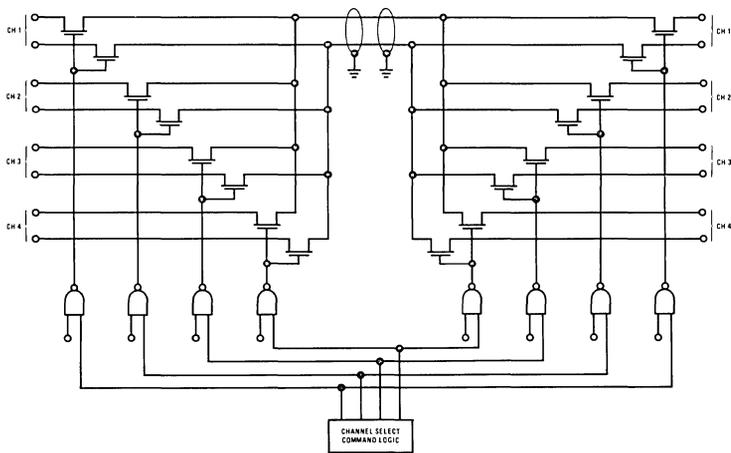
FIGURE 4. Commutation-Modulation and Demodulation
