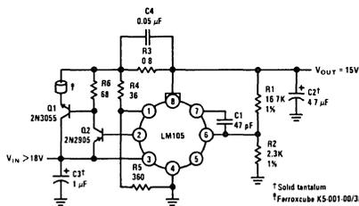
FIGURE 9. 2A Regulator with Foldback Current Limiting.
