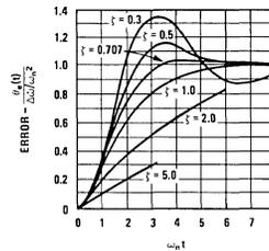
FIGURE 8. Transient Phase Error  $\theta_e(t)$  Due to a Ramp in Frequency  $\Delta\omega$ . (Steady-State Acceleration Error,  $\Delta\omega/\omega_n^2$ , included. Velocity Error,  $\Delta\dot{\omega}/K_V$ , Neglected)
