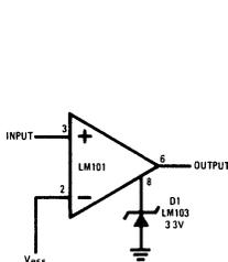
a. Comparator for Driving DTL and TTL Integrated Circuits
