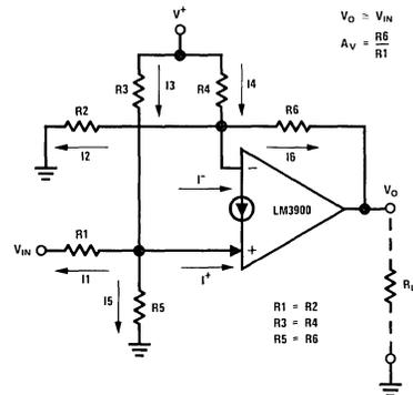
FIGURE 19. A DC Amplifier Employing Common-mode Biasing
