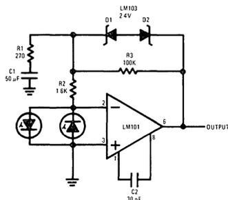
FIGURE 9. Saturating Servo Preamplifier with Rate Feedback
