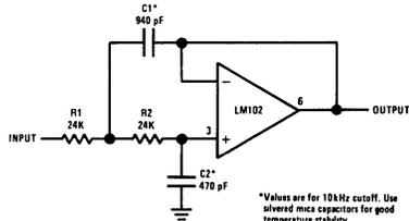
\*Values are for 10KHz cutoff. Use silvered mica capacitors for good temperature stability.
