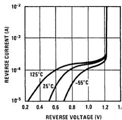
FIGURE 5. Reverse Breakdown Characteristics
