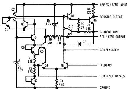
FIGURE 1. LM100 Schematic
