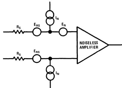
FIGURE 3. Noise Model of an Operational Amplifier
