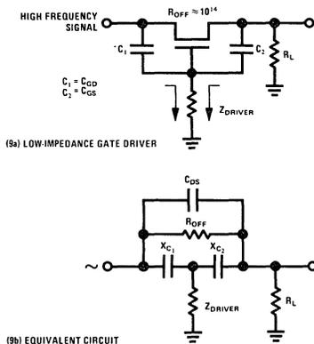
FIGURE 9. Zero-Impedance Driver Return Prevents AC Feedthrough
