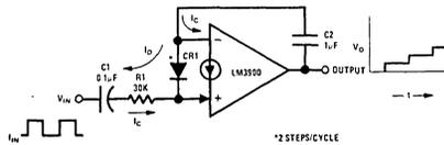
FIGURE 47. Pumping the Staircase Via Input Differentiator
