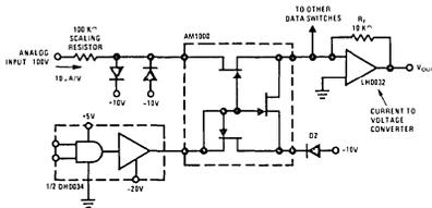
FIGURE 10. Current Mode Multiplexing
