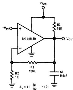
FIGURE 28. Non-Inverting Amplifier
