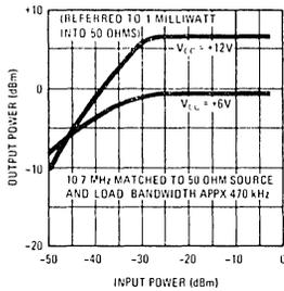
FIGURE 7. Emitter Coupled Limiting Characteristics
