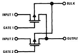
FIGURE 2. Schematic Diagram of Two-Channel Analog Switch.
