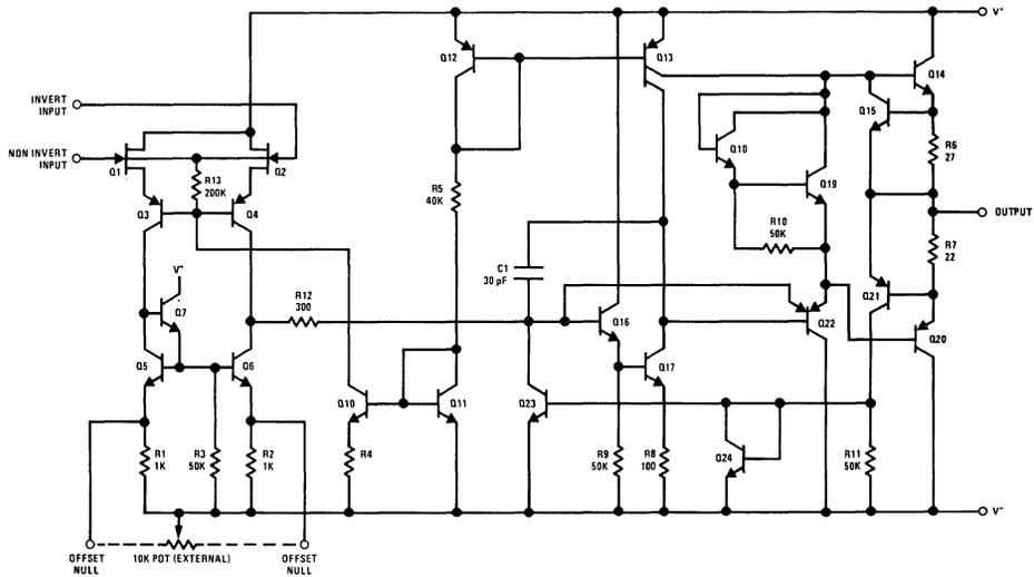
FIGURE 4. Internal Schematic
