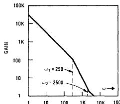
FIGURE 18. Bode Plot for Circuit of Figure 17
