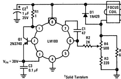
FIGURE 5. Focus Control Current Source
