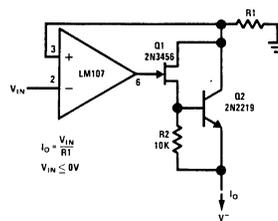
$$I_o = \frac{V_{IN}}{R_1}$$
