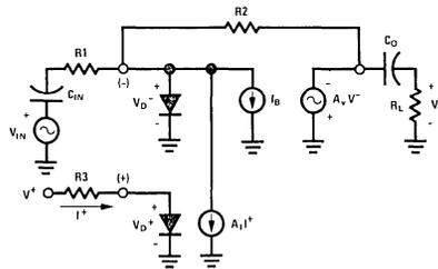
(b) Using the LM3900 Equivalent Circuit
