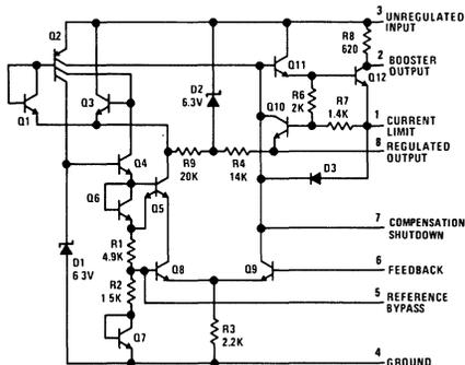
FIGURE 3. Schematic Diagram of the LM100 Regulator.
