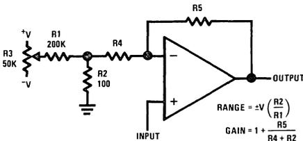
FIGURE 3. Offset Voltage Adjustment for Non-Inverting Amplifiers
