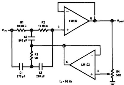
FIGURE 3. Adjustable Q Notch Filter
