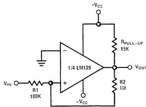
FIGURE 32. Zero Crossing Detector Using Dual Supplies
