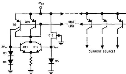
FIGURE 4. Current Source Biasing Circuit
