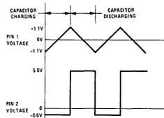
FIGURE 13. VCO Waveforms
