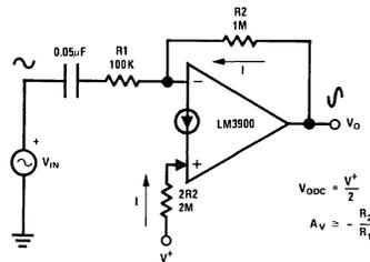
FIGURE 12. Inverting AC Amplifier Using Single-supply Biasing
