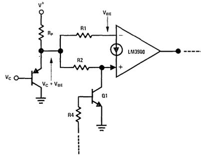
FIGURE 52. Reducing Temperature Drift
