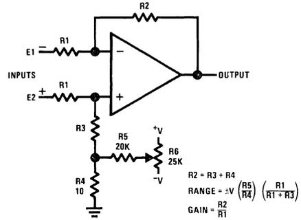
FIGURE 5. Offset Voltage Adjustment for Differential Amplifiers
