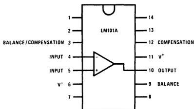
NOTE: Pin 5 connected to bottom of package.
