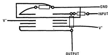
FIGURE 9. Flat Pack Inverting Amplifier PC Layout
