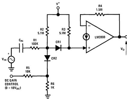
FIGURE 17. An Amplifier with a DC Gain Control
