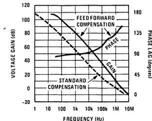
FIGURE 2. Open Loop Voltage Gain
