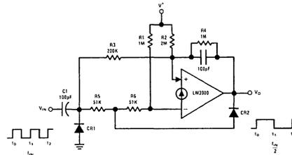
FIGURE 60. A Trigger Flip Flop
