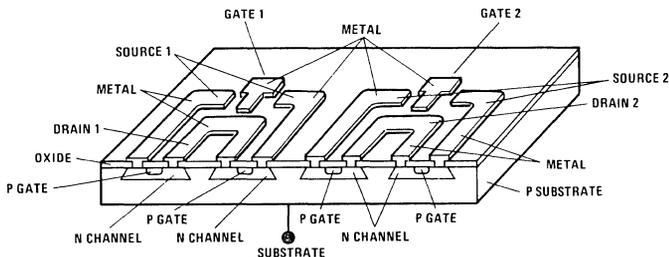
FIGURE 1. Simplified Section of Monolithic JFET Dual
