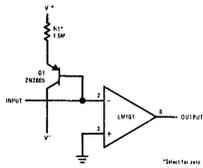
**FIGURE 3. Summing Amplifier with Bias-Current Compensation.**
