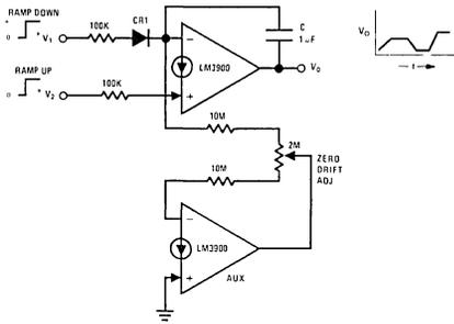
FIGURE 85. A Low-drift Ramp and Hold Circuit
