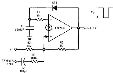
FIGURE 65. A One-amplifier One-shot (Negative Output)
