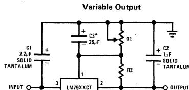
\*Improves transient response and ripple rejection. Do not increase beyond  $50\mu F$ .
