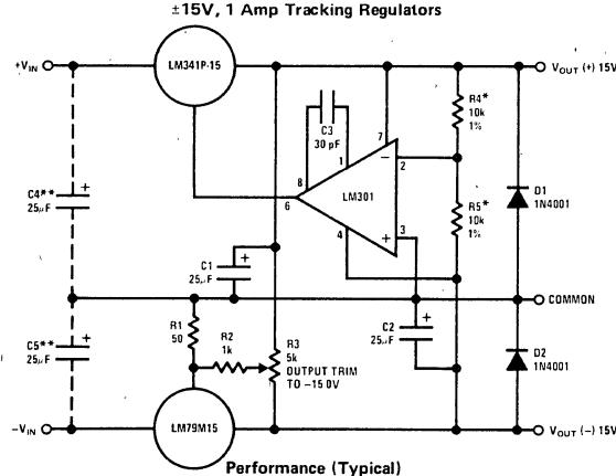
\*Resistor tolerance of R4 and R5 determine matching of (+) and (-) outputs
